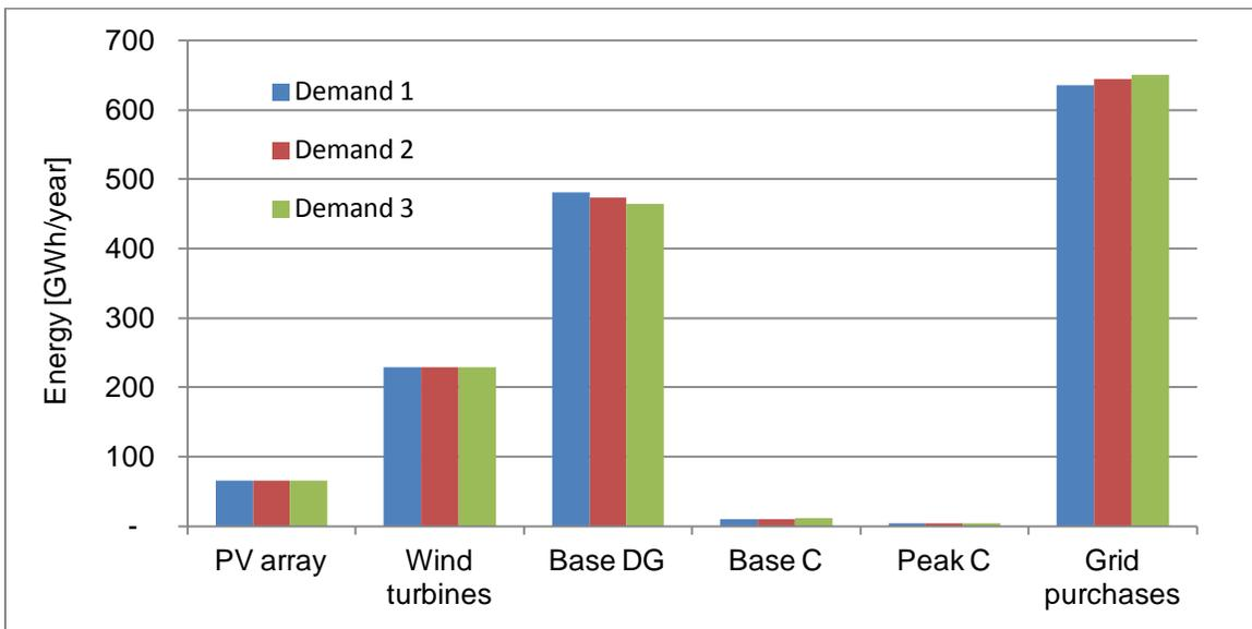
Change in demand will cause different energy production by different generators. This will also affect capacity factor (Exhibit C - 17) and number of operating hours (Exhibit C - 18).
