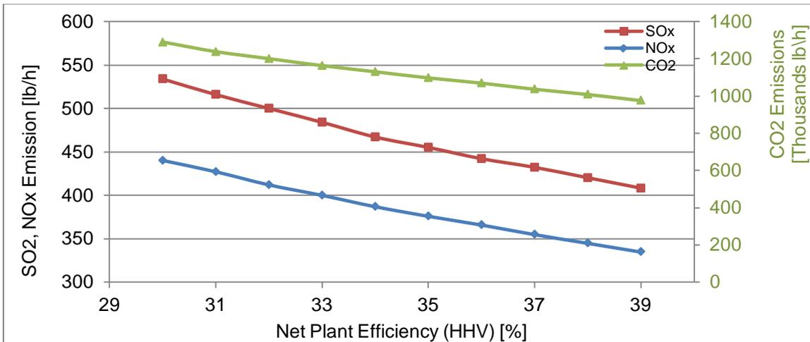
Note: Supercritical PC without Carbon Capture, CF=85%; Net Plant Output 550 MWe
