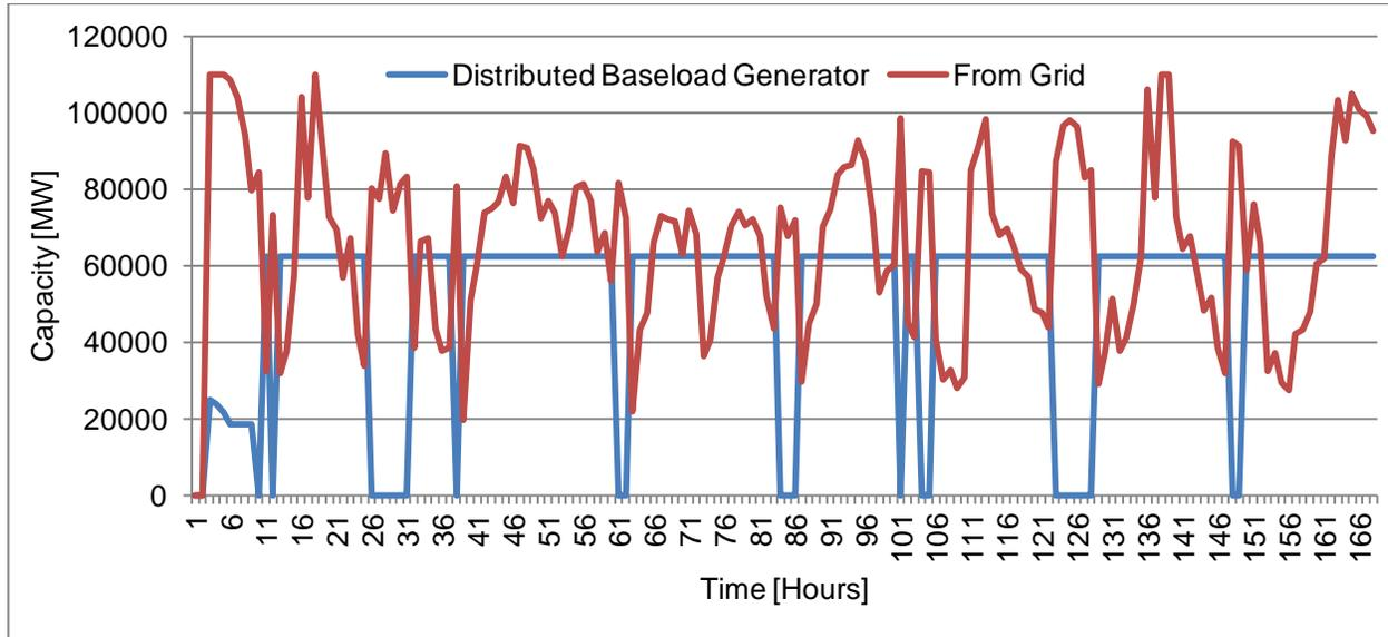
The given examples illustrate distributed baseload generation behavior for three different ways of buying 45 percent of annual energy for Smart Grid city’s energy consumption from the grid. If the distributed baseload generation is not capable of load or wind/solar fluctuation following, additional back-up power from the grid is needed to firm up renewable generation.
