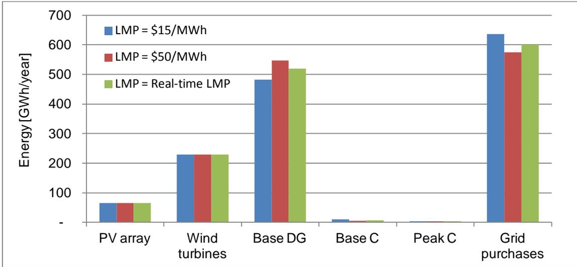
Base DG will produce 480 GWh if LMP is \$15/MWh, about 550 GW if LMP is \$50/MWh and 520 GWh if LMP is real-time LMP. Different Base DG will be compensated from the grid such
