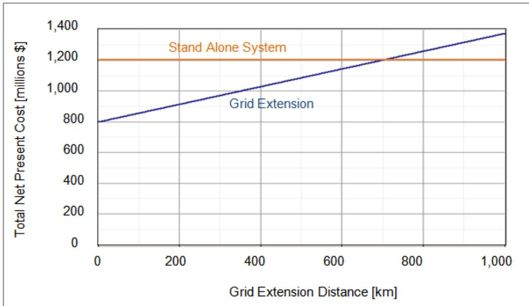
Key assumptions in the above analysis include the calculation of capacity factor as number of operating hours divided by 8760 hours, and, maximum and average demand are used in the calculation instead of demand curve. Both assumptions are valid for the first level of economic
