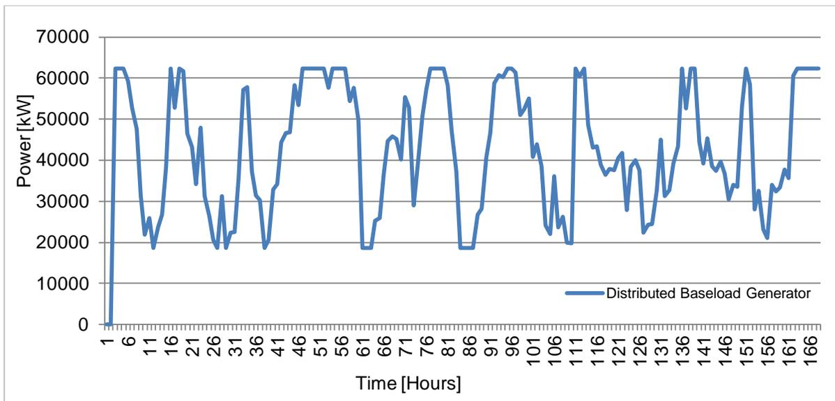
The baseload distributed generation compensates for wind and solar fluctuations (Exhibit C - 4). The generator is used 8,760 hours per year and its capacity factor is 77 percent. If the generator is not capable of fast ramping up and down, it should be accompanied with storage or additional backup power should be supplied from the grid.
