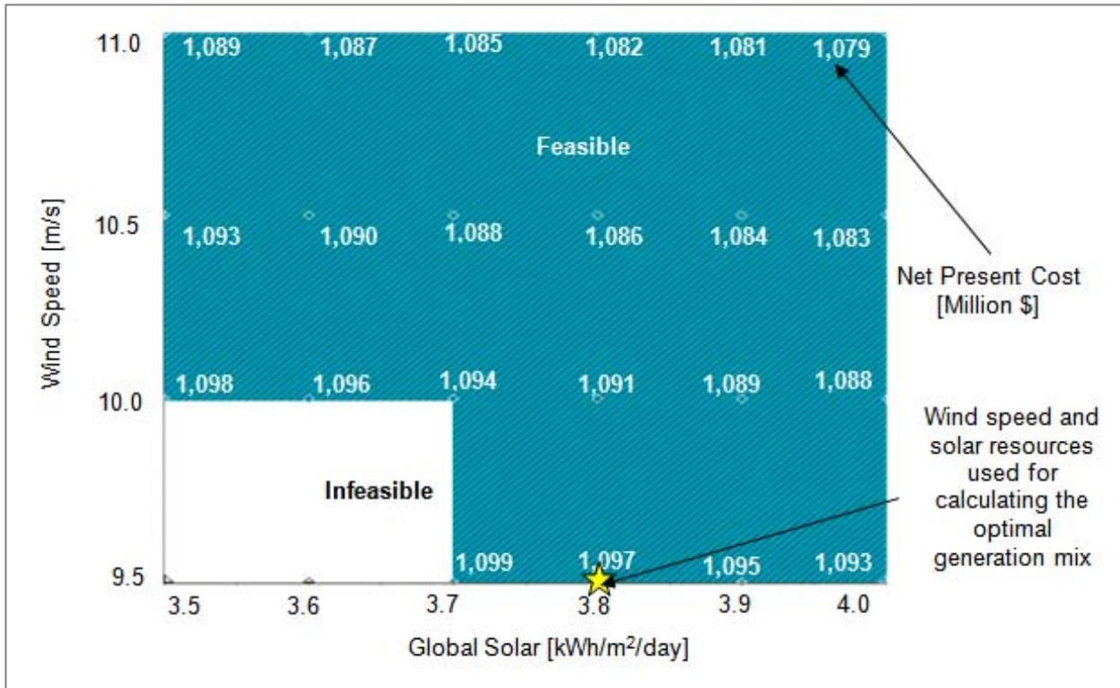
The set of feasible solutions increases if wind generation capacity can increase to 60 MW. Exhibit C - 8 illustrates a sensitivity analysis for this case. The optimal generation mix will not contain PV generation if wind speed increases above 10 m/s. The optimal generation mix will be infeasible if wind speed drops below 8.5 m/s and solar resources drop below 3.0 kWh/m<sup>2</sup>/day.
