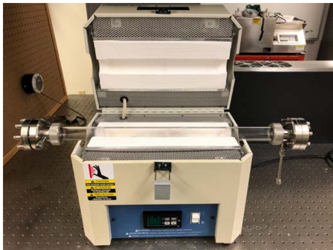
Tube furnace used to pyrolyze samples
