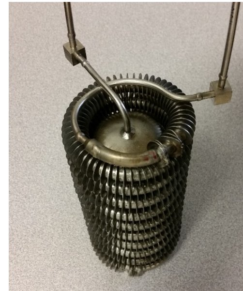
Coiled-fin tube exchanger in CHEX between dual AMRs
