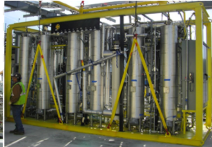
TDA 0.1 MW pre-combustion carbon capture unit installed at the National Carbon Capture Center
