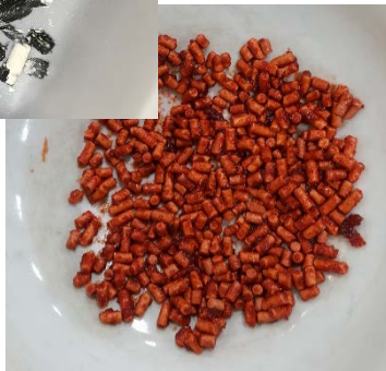
Insufficient coating thickness
