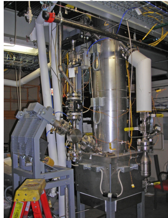
Figure B-4. Design drawing of the pressurized, fluidized-gasification reactor.
