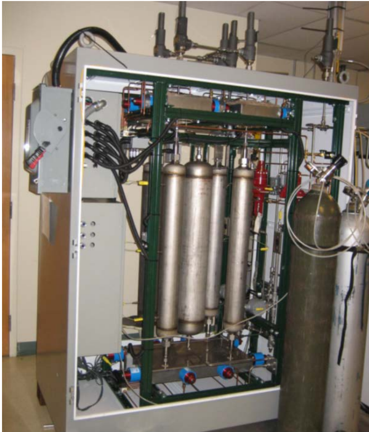
4-bed PSA Skid
