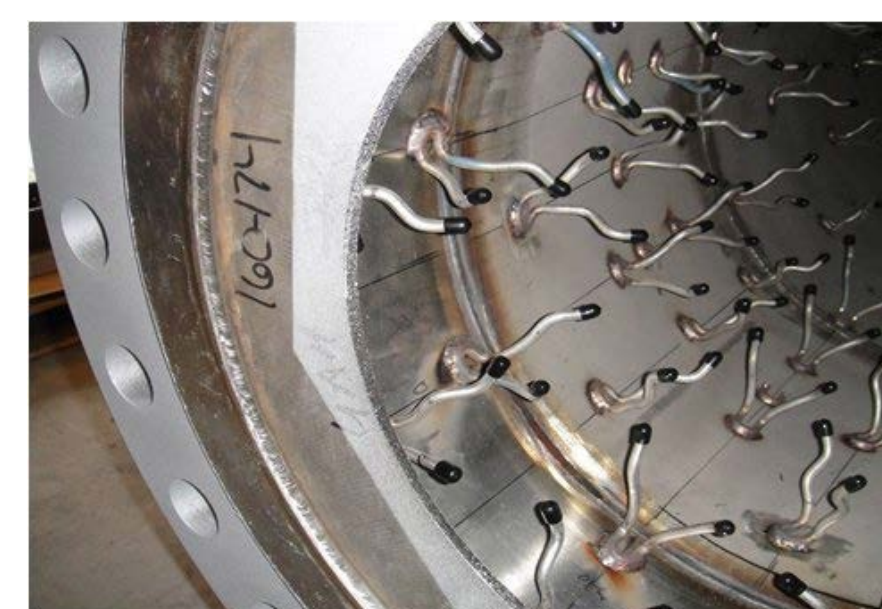
Anchors (left, image from TFL Houston) might be installed using powder feed or wire feed AM, while gunning (right, image from Kiltas) might be controlled via robotics.
