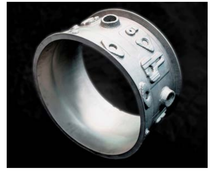
Hybrid manufacturing building CAD/CAM-enabled three-dimensional structures on existing metal pre-forms made using traditional metal forming methods. (Image from DM3D Technology)
