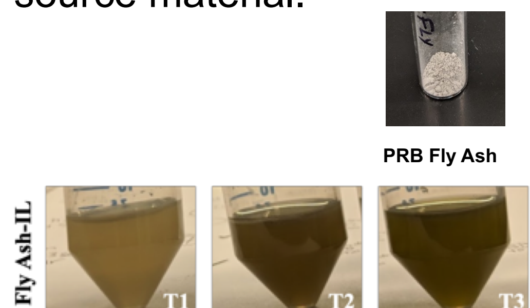
Figure 4. Dissolution of fly ash into IL varied by treatment conditions. Fly Ash/IL solutions.
