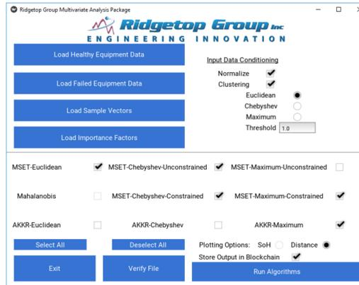
Figure 7. Prototype software program for the Multivariate Analysis Package. In Phase II Ridgetop Group intends to import this software analysis package into the Sentinel Suite cloud platform for advanced diagnostics and condition based maintenance.
