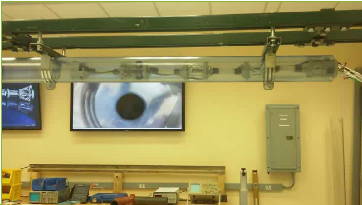
Pipe crawler allows for inspection without disassembly.
