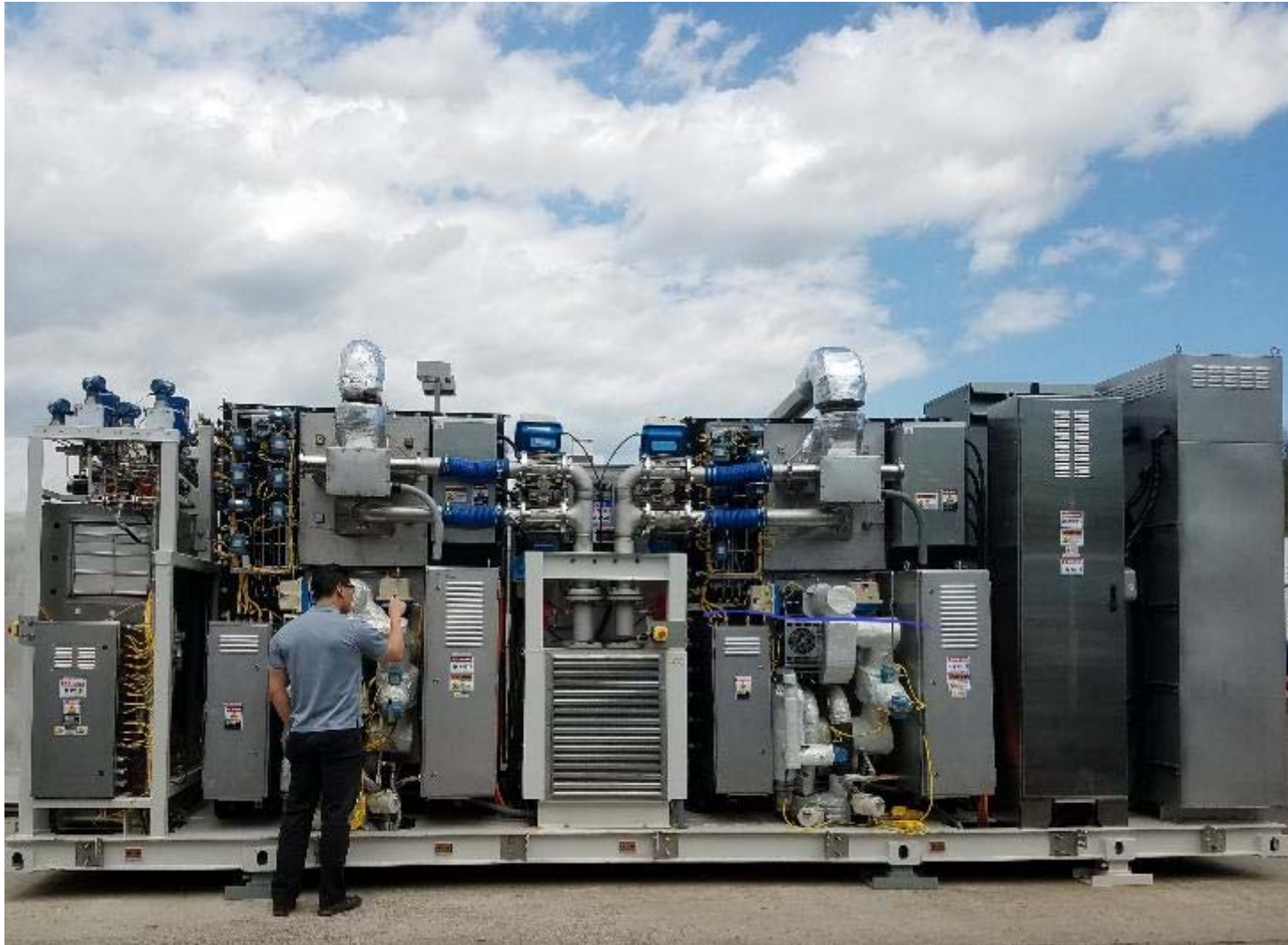
200 kW system installed at FCE's Danbury, CT Test Facility.
