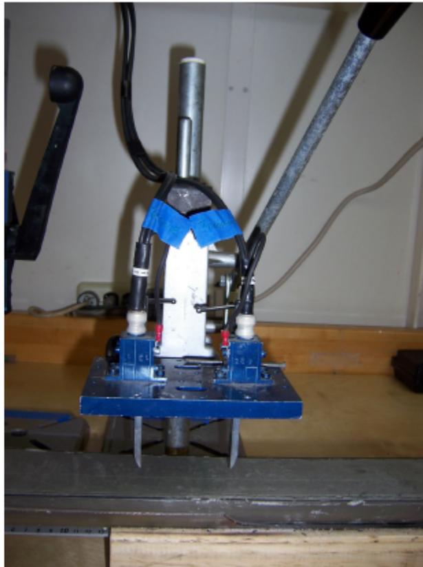
Figure 10 – *P*-wave Measurement System
