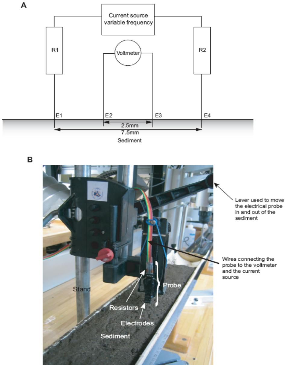
**Figure 9 – Electrical Resistivity Measurement System**
