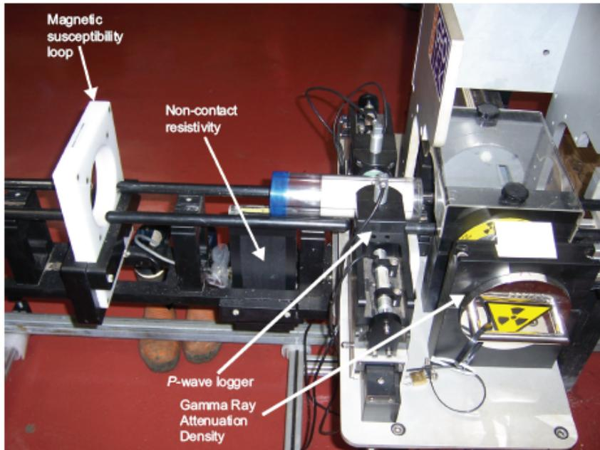
Figure 8 – MSCL-S System mounted on Track
