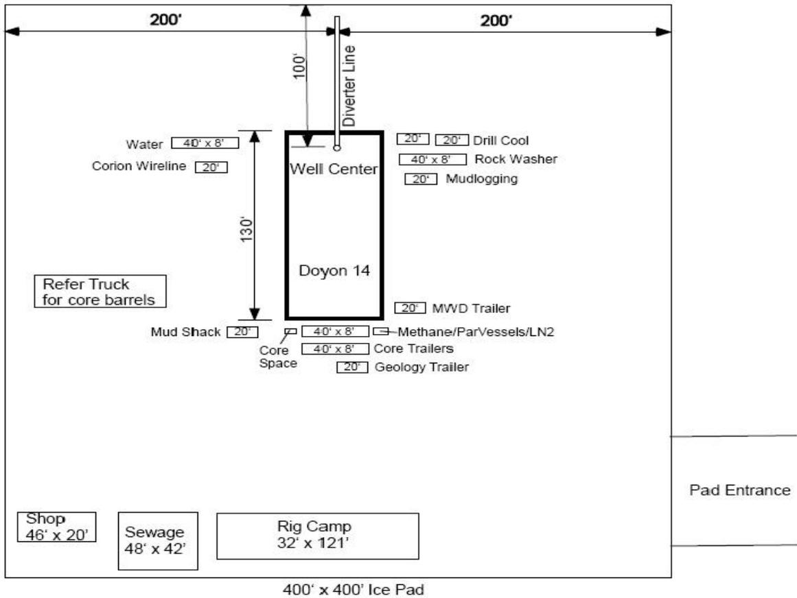
Figure 5: Ice Pad and Rigsite layout diagram. Note that Rig Camp and facilities will likely be staged on MPB-pad, approximately 1 mile to the north.
