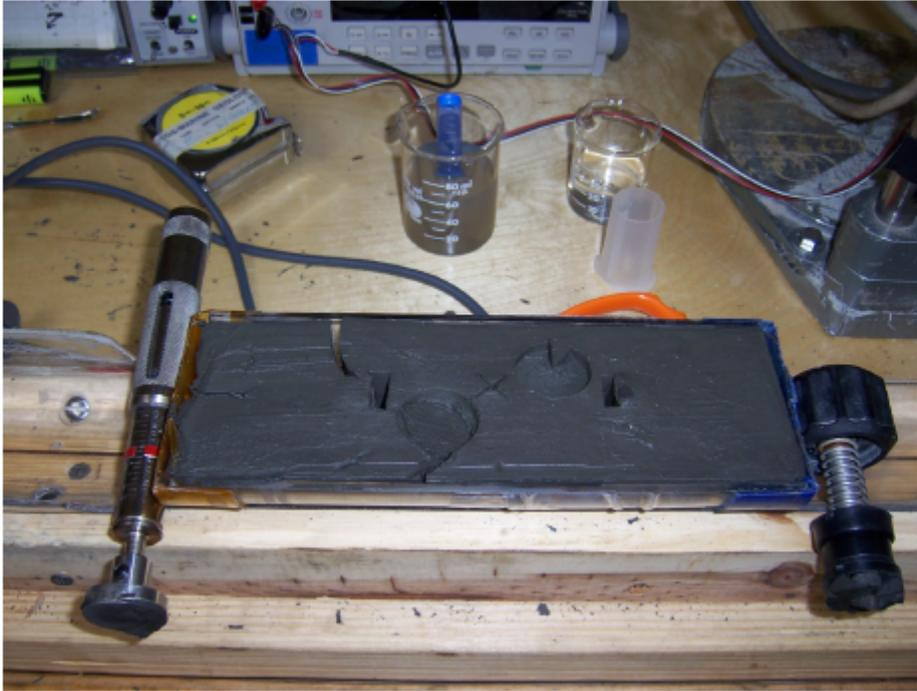
**Figure 14 – Pocket Penetrometer**
