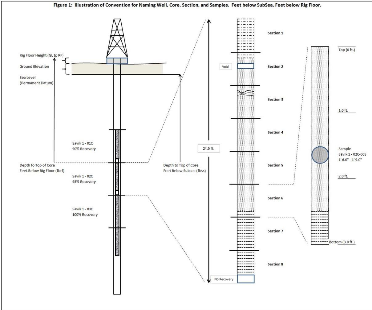
**Figure 1 – Conventions for noting holes, cores, section, and samples, with depths**
