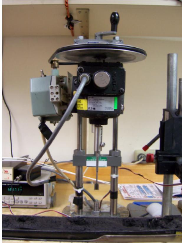
**Figure 11 – Mini-vane Shear Machine**
