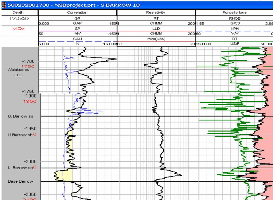
Figure 3: East Barrow Type Well (S. Barrow No. 18), Showing Anticipated Core Interval
