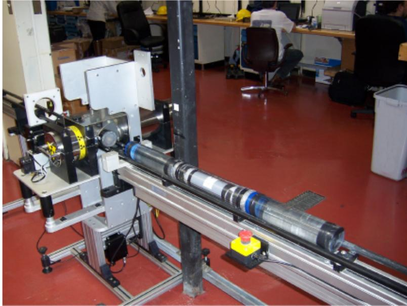
Figure 7 – MSCL-S System mounted on Track
